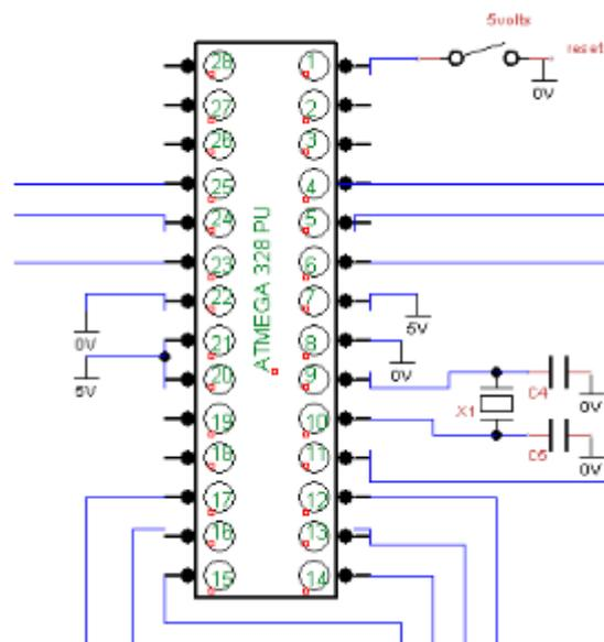
**Fig 1.3: ATMEGA 328 PU unit**
