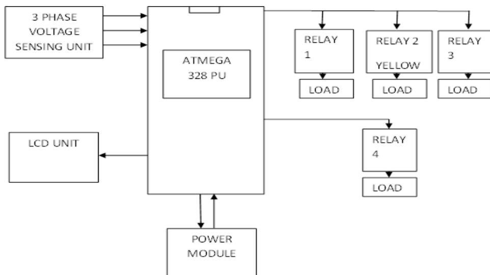
Figure 1.1: Block diagram of Automatic Phase Selector and Changeover Switch
