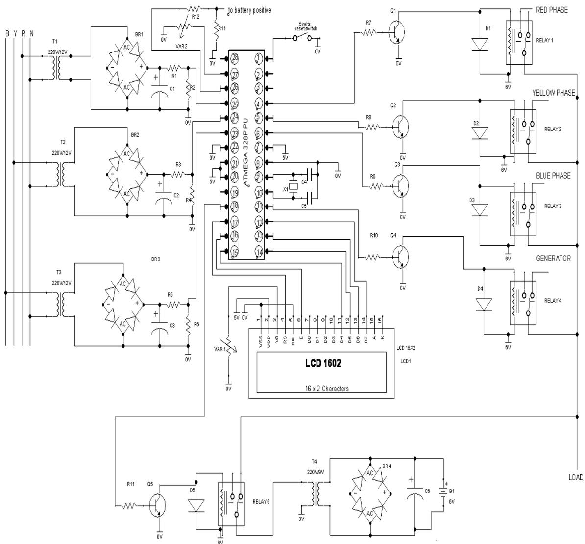
Fig. 1.7: Circuit diagram of the Automatic Phase Selector and Changeover Switch
