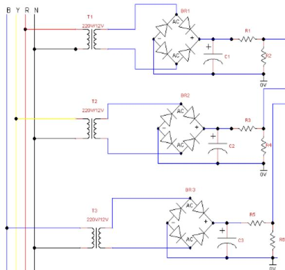
**Fig. 1.2: Circuitry of 3-Phase Sensing Unit**
